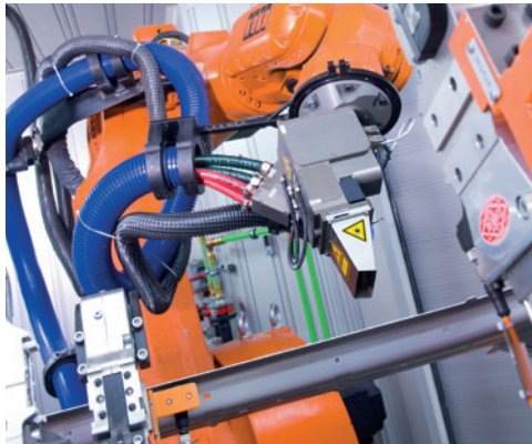
cleanLASER during welding pre-treatment in body-in-white production
